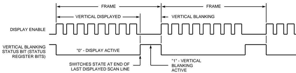
Figure 8. Operation of Vertical Blanking Status Bit
