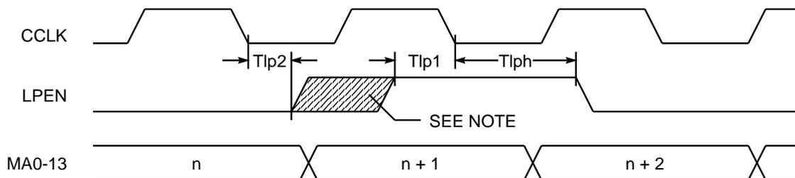
NOTE: "Safe" time position for LPEN positive edge to cause address n+2 to load into Light Pen Register. Tlp2 and Tlp1 are time positions causing uncertain results.
