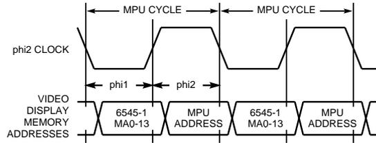
Figure 6. phi1/phi2 Interleaving
