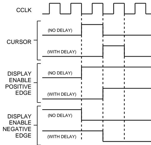
Figure 7. Cursor and Display Enable Skew
