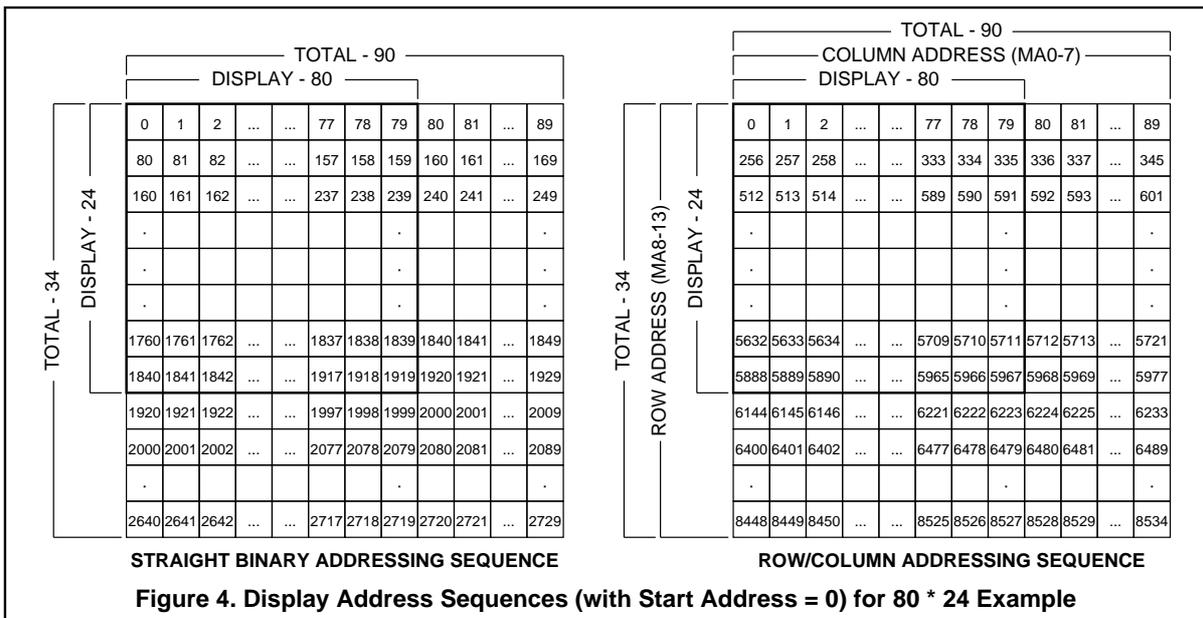
**Figure 4. Display Address Sequences (with Start Address = 0) for 80 \* 24 Example**
