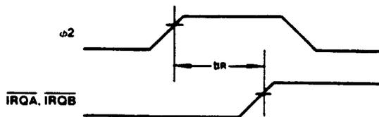
Figure 11. Interrupt Clear Timing
