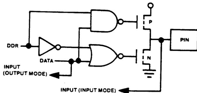
Figure 15. Port B Buffer Circuit (PB0-PB7)
