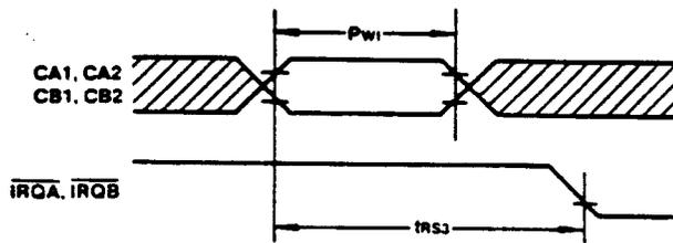
Figure 10. Interrupt Timing
